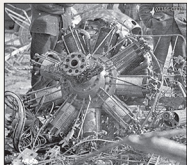
The Bentley BR.1 engine and some steel tube framing is almost all that remains of this Sopwith Camel that was reportedly destroyed by a bomb. Note the tell tale 'nonagon' crank case and cylinder fixing bolts which are the most obvious differences between the Br.1 and Clerget engines.
