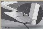
Fin and rudder detail from an unidentified Ruston & Proctor built Sopwith F1 Camel.
