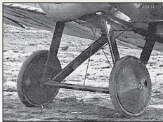
Fabric wrapped tube steel & wooden fairing undercarriage from an unidentified Sopwith F.1 Camel. Sopwith Camel undercarriage struts, especially the port side, were perennially soaked in castor oil which spewed out from the engine. Remarkably, a problem with the port wheel unscrewing itself and falling off(!) was not fixed until May 1918 when opposite thread bolts and axles became available. Note the Palmer Detachable Shield No.2.
