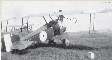
This unidentified Sopwith built F.1 Camel was photographed at Lympne in August 1917 and, although unconfirmed, was probably powered by a 130hp Clerget 9B engine. Note the factory applied stencilling on the side of the fuselage, fin, horizontal tailplane and elevator. The struts and ply fuselage panels are stained dark brown while the aluminium cowlings remain unpainted.
